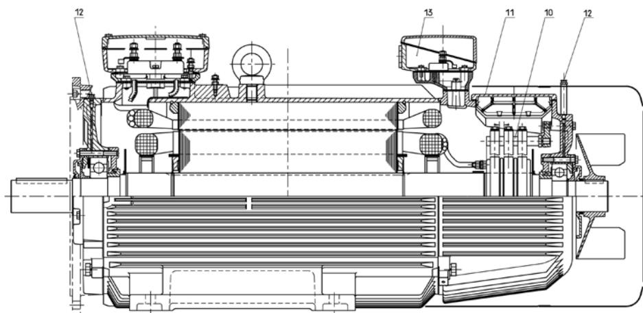
Figure 2: Mechanical design of slip-ring motor S11R/S11H 315 MX-LY
