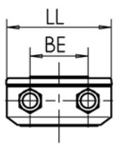
Standard terminal box for screwed cable glands
