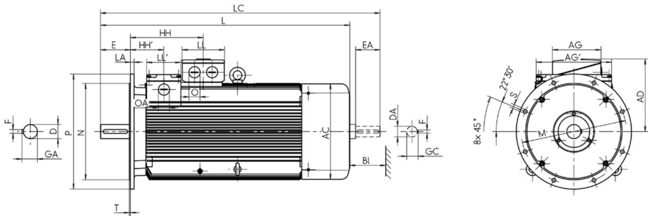
Type of construction IM B5K [IM 3003], IM 3004; up to size 200, IM V1K [IM 3013], IM 3014
