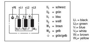
Three-phase asynchronous motor Delta connection
