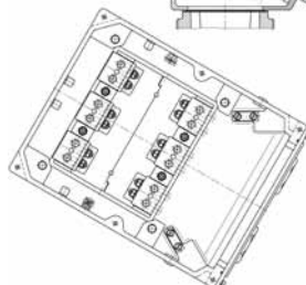
Figure 07S Terminal box 1000 A, Ex eb IIC inclined intermediate flange
