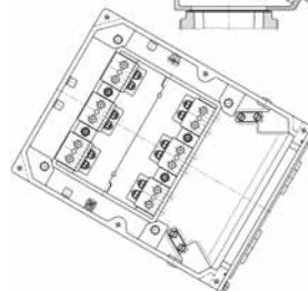
Figure 04S Terminal box 1000 A, inclined intermediate flange
