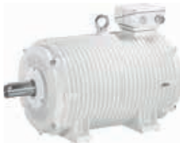
ARC 400 LX8 LL TPM HB IL HW 60 kW, rullaratamoottori
