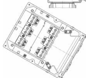
Figure 07S Terminal box 1000 A, Ex eb IIC inclined intermediate flange
