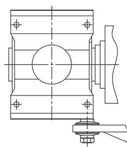
All units can be supplied with elastic constraint, semi-flexible and rigid reaction arrangement.
