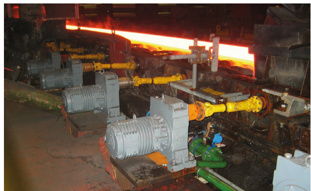
Figure 6: Delay table with S141-1A ARG 160L 4, M_{max} = 1039 \text{ Nm}
